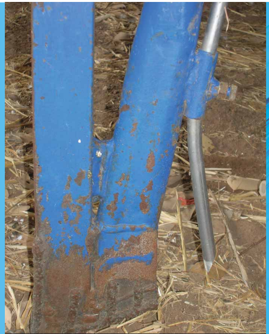
Liquid inject point behind the tyne openers
